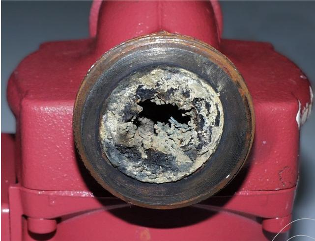
A magnetic filter can only collect the debris that passes within a few centimetres of the magnet, and so without the assistance of a vigorous flow rate generated by a power flushing pump, accumulated deposits will remain static within radiators and pipe work, continuing to diminish the efficiency of the system.
