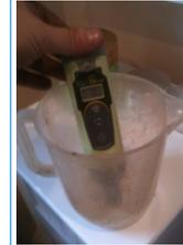
Whilst the water is being dumped from each radiator, a sample of water is taken. This sample reading must match that to the incoming mains water to ensure that the system is cleaned effectively.
